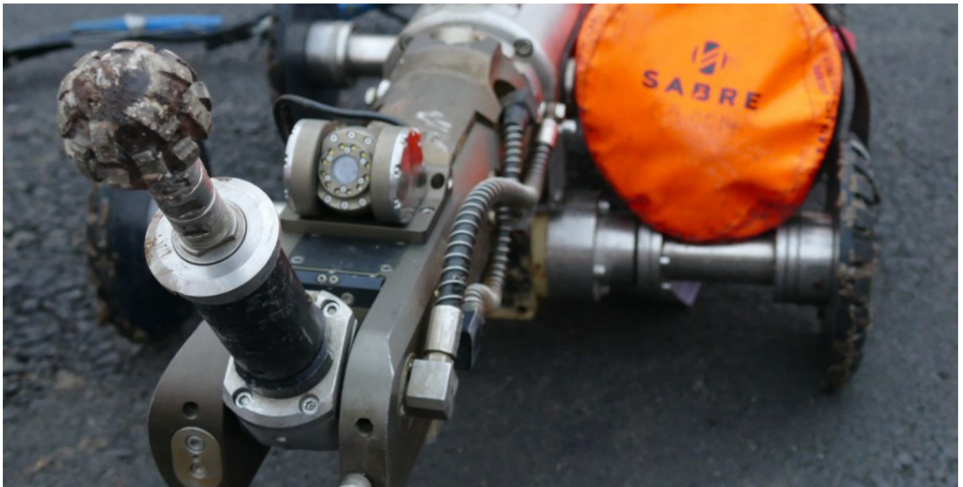
A robotic cutter used in sewer rehabilitation.
