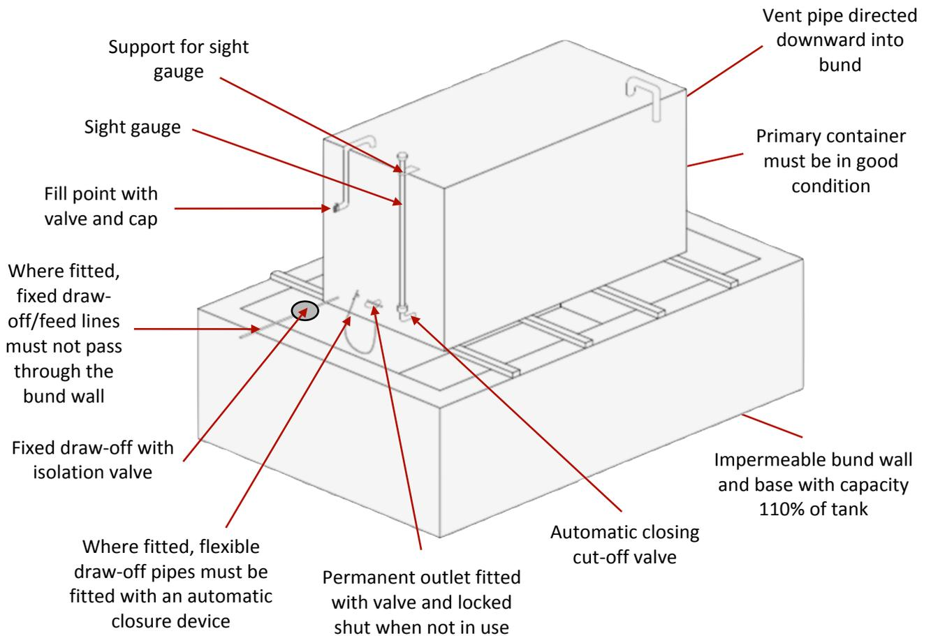
**Figure 2: Totally Enclosed Bunded Oil Tank**
