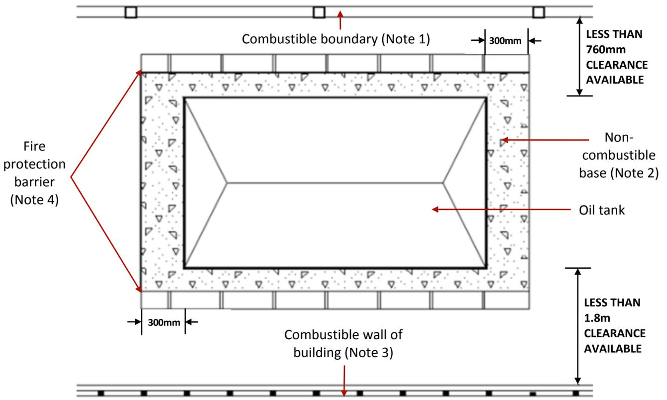
**Figure 5: Oil Tank Installation Near Non-Combustible Buildings & Boundaries**
