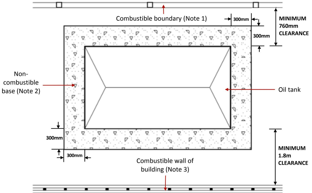
**Figure 4: Oil Tank Installation Near Combustible Buildings & Boundaries**
