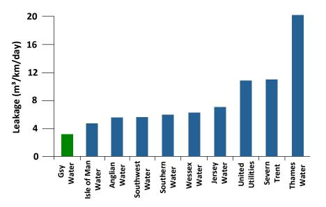
To put the leakage figures in perspective, the graph on the left shows Guernsey Water's leakage figures (represented as cubic metres per kilometre of main, per day) against the figures from a number of other water companies. Please note that 2009 figures are used for the other companies as not all 2010 figures were available. However, they give a good comparative indication.
