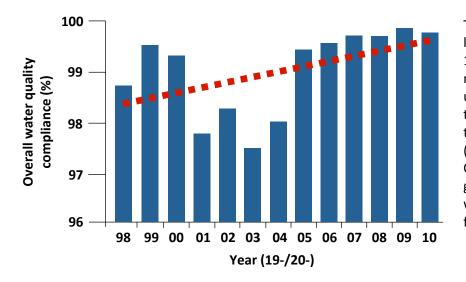
The red dotted line represents the linear trend over the period from 1998 to 2010. With the Island's two main water treatment plants now utilising state-of-the-art membrane technology, and improvements taking place at service reservoirs (e.g. through the installation of OSEC - Onsite Electrolytic Chlorine generation plants), it is hoped that water quality figures will increase further in the future.
