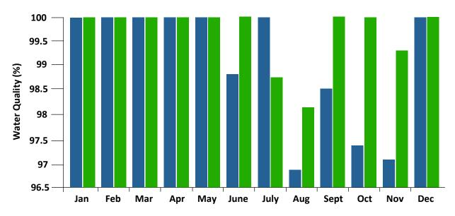
The graph shows the expected pattern of water quality dropping slightly during the warmer summer months when air temperatures increase, which can lead to bacteriological growth.
