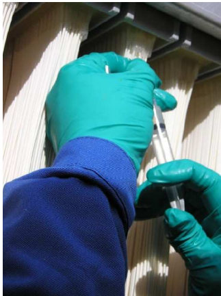
Filaments being checked by hand
